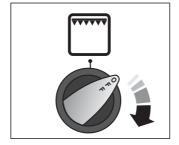
The broiler has two elements that allow either the whole area of the pan to be heated or just the right hand half.
